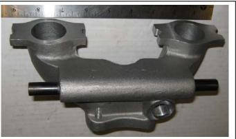
Suitable for HS4 (1 ½"), HS6 (1 ¾"), HIF4 (1 ½"), or an HIF6 (1 ¾") carburetor. The larger ports make this manifold ideal for large capacity engines (1380cc. for example). There may be hood clearance issues with a Bugeye, but we do not have any known examples of the problem to support this theory.
