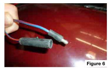
Note: The original wires going to the low beams and to the high beams each split so they can feed both sides of the car. You need to connect the wires from the relays with the male bullet connectors upstream from that split. If you don't, only one side of the car will light.
