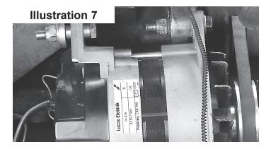
If the wires removed from the generator are fitted with the ring type connectors then the female spade connectors will have to be installed. To do so, remove the ring type connectors with wire cutters and strip 1/4" of insulation off of each wire. Attach one of the two non-covered female spade connectors to the Brown/Yellow wire and a small red spade connector to the Brown/Green wire using wire crimpers. Use a 1" section of the heat shrink provided to cover the larger spade connector.
