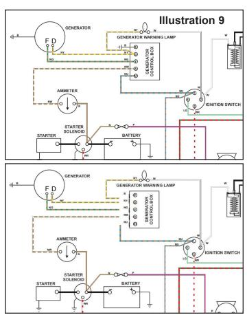
10. Plug the wires into your alternator as shown.
