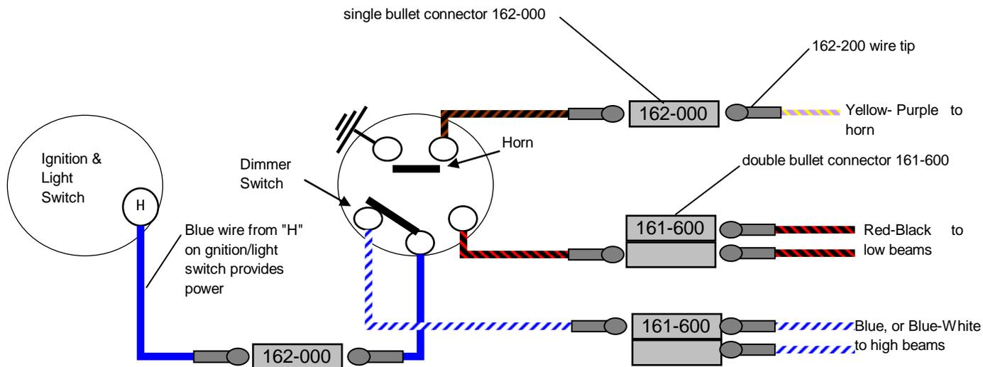
The schematic above shows how the switch can be connected.
