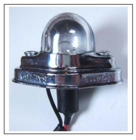
This lamp assembly includes the socket with wires, bulb, gasket for glass dome, glass dome, chrome hood, and screws that secure the chrome hood to the lamp base.
