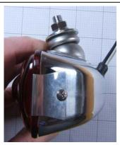
If the wires must pass through the body shell, use an existing grommeted hole, or drill a new hole and use a suitabel grommet. The wiring may be spliced directly into the main harness in the car, or you may use existing bullet connector blocks if suitable witre tips are soldered onto the wires. We suggest 162-200 wire tips if you choose to go that route.
