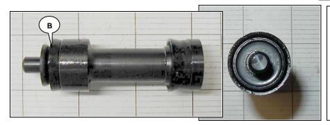
Type 2 piston, as found in AP Lockheed master cylinders made from 1995 to 2003, and AP master cylinders from Aug 2008 on.
