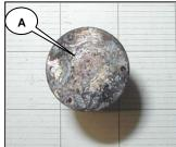
Type 1 or "OE" style piston, as found in Lockheed master cylinders made prior to 1995. Also found in some older aftermarket master cylinders. Cup type primary seal sits on the end of the piston (A).
