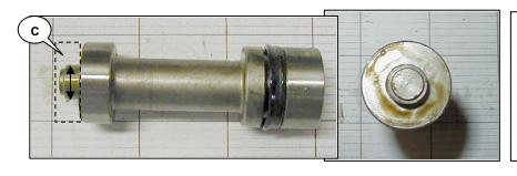
Type 3 piston, as found in Lockheed-Delphi master cylinders, made from 2003 to about Aug 2008. Ring type primary seal (C) has been removed to show end of piston.
