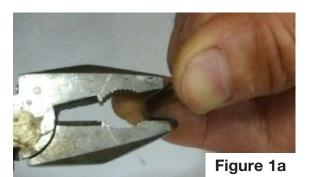
Squeezing clip tighter to increase tension
