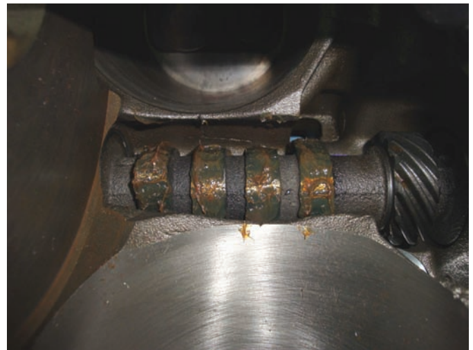
figure 7 - Lubricant #4 on Cam Lobes #15 & #16
