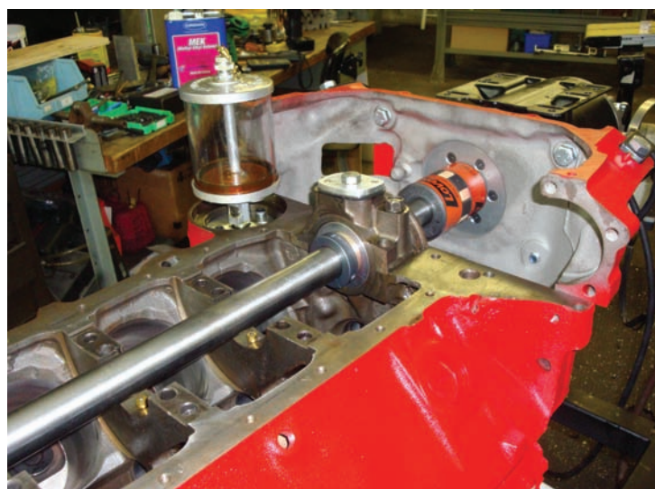
figure 2 - Drive Shaft and Plugged Main Bearing Oil Holes
