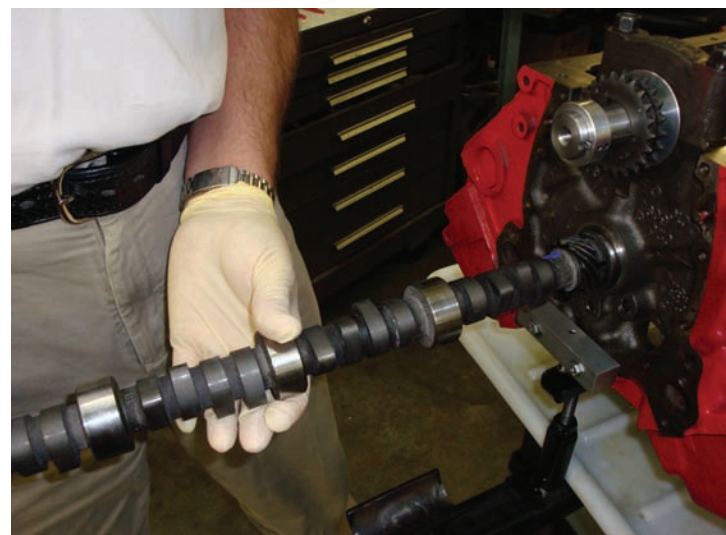
figure 3 - Clean and Dry Camshaft Installed into Bore
