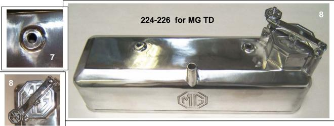
Note that the filler for this valve cover is always to the rear, even on the MG TD. Clausager, in his <u>Original T</u> Series, has a nice picture of an original alloy valve cover on a TC on page 26.
