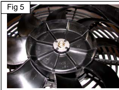
Fig 5 Flip the fan over so you can see the nut.
