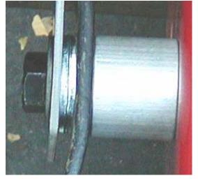
With or without the washers, the rack should look like this before we begin to attach the arms to the upper mounting points. The large bolts that secure the bumpers are snug, but not real tight. We just need to keep the rack from moving around too much side to side as we attach the arms.
