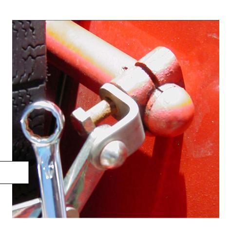
91 The driver's side or LH side pinch bolt is harder to get to because of the license plate.
