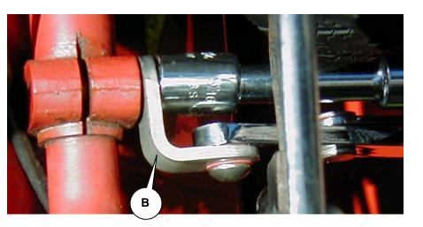
On the passenger's or LH side, you have easier access. You can easily slip an adjustable wrench on the bracket. That makes it easy to hold the bracket still as you tighten the pinch bolt.
