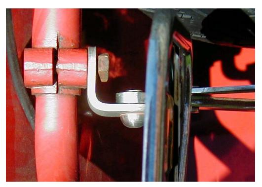
At this point, all four bolts – the two lower bumper bolts, and the two upper pinch bolts, are in, but not tight.
