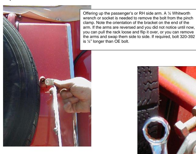
Threading the bolt back into the clamp
