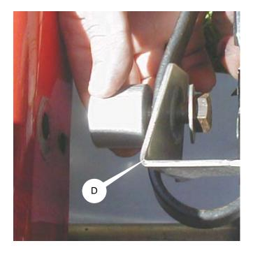
Here you can see the driver's or LH side bolt installed, but still loose. Both sides need to be loose.
