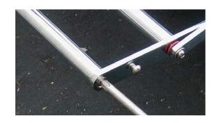
Tighten up the phillips head screws that hold the sides of the rack to the tubing.
