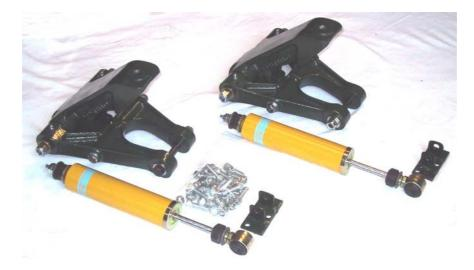
The conversion kit consists of a pair of precision-machined aluminium wishbone and damper mounting units, HBE gas telescopic dampers, lower damper mounting brackets and a fitting kit.
