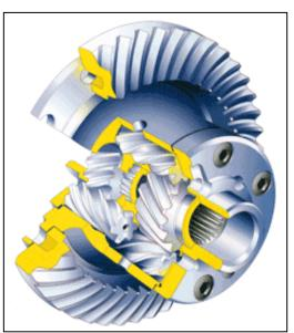
The Quaife torque biasing differential enables your car to accelerate quicker and corner faster. How?
