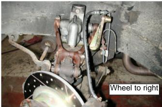
**13.** Remove the nuts and lock washers on the end of the two bolts on the rear face of the lower spring pan. Use a 1/2" combination wrench and a 1/2" socket. **DO NOT** remove the bolts. If you do remove the bolts, you must fully support the spring pan with a jack, or the suspension spring may bend the spring pan or break the front spring pan bolts.
