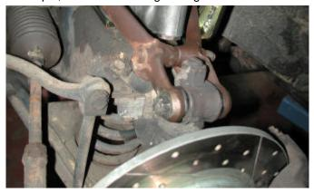
11. Use an adjustable wrench to attach the supplied brake hose to the supplied brake hose extension labelled 181-225. Use a small adjustable wrench to disconnect the brake hose from the hard line at the body. Then, attach the hard line/soft hose with the loop at the bottom and the S-curve at the top doglegging rearward, away from the steering rack. The picture shown is of the car's left side. Try to match the angle/orientation.
