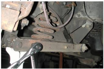
**14.** Slide the new lower shock bracket (the lowers are the same) over the two bolts in the lower spring pan with the shock stud parallel to the hole in the upper shock mount. Slide on the factory lockwashers. Thread on the provided 5/16-24 nuts and tighten them to 18 ft-lbs with a 1/2" socket.
