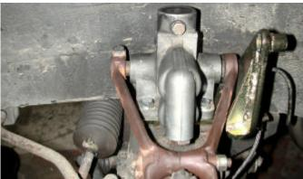
**10.** With the lever arm (Armstrong) shocks bolted down, retorque the bolt and nut at the end of the upper A-arm to 30 ft-lbs. Note: this bolt should not be too tight, as that will restrict the movement of the arm. If there is a cotter pin, reinstall it after tightening.
