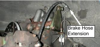
**12.** Attach the rubber brake hose to the metal brake hose extension. Working on the left side, give the brake line a slight clockwise twist so that it will clear the wheel with the steering wheel turned all the way to the left or all the way to the right. Attach the line to the brake caliper but do not tighten the crush washers. You will readjust the twist in the brake line for clearance later.
