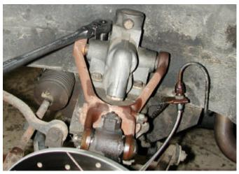
**3.** Pull the A-arm so that the shock sits upside-down and the large damper valve retaining bolt is accessible. Either hold the spindle and brake caliper in place or
