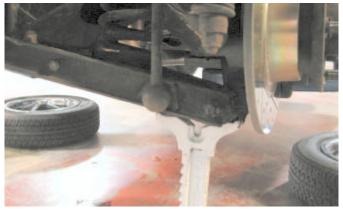
**2.** Use a 9/16" deep socket and a ratchet to remove the **four** bolts holding the lever arm shock to the cross-member. Alternatively, a 9/16" socket and a short extension could be used.
