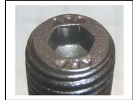
**IMPORTANT! DO NOT TORQUE THESE STUDS INTO THE BLOCK AT 35 lbs-ft as specified in the workshop manual!** If you do, you will crack the block because there is a water gallery within a ½ inch of one of the studs, and the unthreaded section of the stud has a chamfered shoulder which acts like a wedge. **Install the studs into the block finger tight.**
