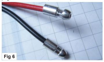
The 10 amp fuse (7a) OE part number 27H5903, or Moss Part Number 146-730 is included. Note that the tinned terminals are solidly crimped onto the wires and the insulation.
