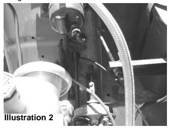
**3.** Now, find a source for the boost/vacuum gauge. The source should be between the carburetors and the cylinder head or between the supercharger and the cylinder head. If your car is naturally aspirated, find a spot in the intake manifold that you can tap into or find a spot to drill and tap to 1/8" NPT (the tap drill for 1/8" NPT is an "R" drill). Be sure to remove the intake manifold from the engine before drilling to prevent metal chips from entering your engine. Note: The location
