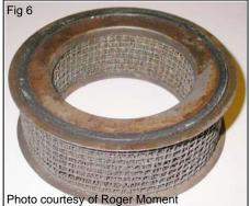
The 372-040 Coopers Type filter element will fit into the Burgess housing, and makes a reasonable vintage looking replacement.
