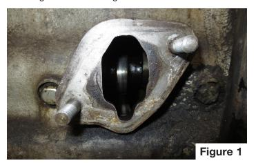
2) Before installing the fuel pump on the engine, the engine must be rotated so the cam shaft is in a suitable position to accept the pump. Out of 720 degrees of crank shaft rotation (2 full turns) only about 180 degrees are suitable for fuel pump installation.
