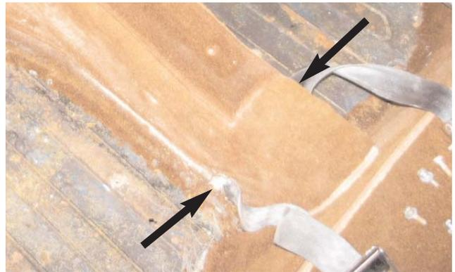
9. Pull up the carpet covering the top and sides of the center console area up to where the rear of the center console was separated from the front. The shift lever will keep the carpet from being pulled farther forward. Then pull up the carpet on the sides of the center console in the footwell area. There may be a factory aluminum heat shield in this area. If so, leave it in place. There is a separate piece of carpet behind the emergency brake. This should also be left in place.
