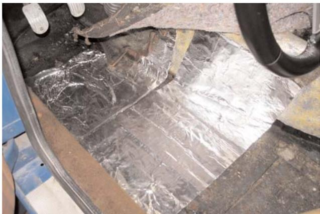
**15.** Gather the two “almost square” sheets that resulted from cutting a insulating material sheet in half back on **Step 3**. Apply one “almost square” insulating material sheet onto the toeboard on each side of the vehicle. Again, take note of any carpet retaining snaps on the floor that will be
