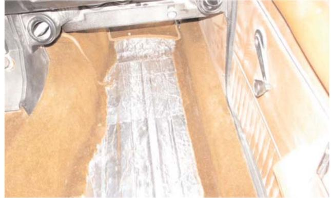
**20.** Spray the carpet contact adhesive onto the top of the transmission center console in between where the seats mount. Then lay the carpet down and press into place.
