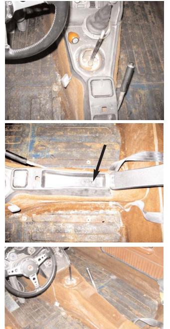
**7.** Remove the fiber spacer that is on top of the carpet surrounding the shift lever.
