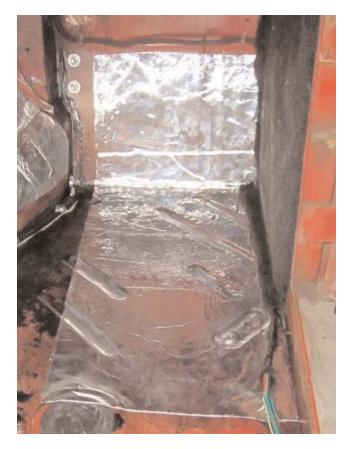
**12.** You will notice that there is a strip of floorboard between the edge of the Hushmat sheet and the transmission tunnel cover. This strip will be covered next. Gather one of the discarded pieces of wax paper backing and the black permanent marker. Lay the
