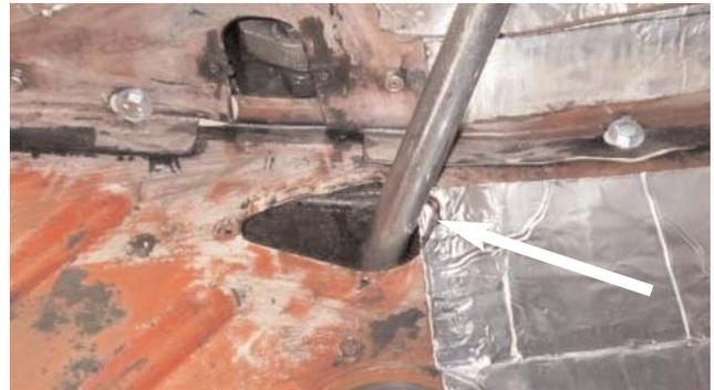
**13.** Now cover the area between the front of the seats and the sheets of Hushmat already applied to the floorboard area. Use the wax paper and the black permanent marker to draw an outline of the area onto the wax paper, cut it out, check the fitment, recut if necessary and install the sheet without the backing. Then use the black permanent marker to mark out the edge of the emergency brake handle hole, the two carpet snaps and the body drain plug hole.
