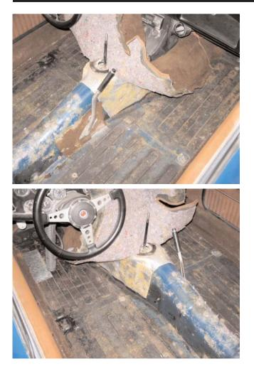
**10.** Pull up just the edge of the carpet that touches the floor on both the left and right side square frame rail at the far left and right sides of the passenger compartment. The sound deadening mat will go **UNDER** the carpet here when installed.
