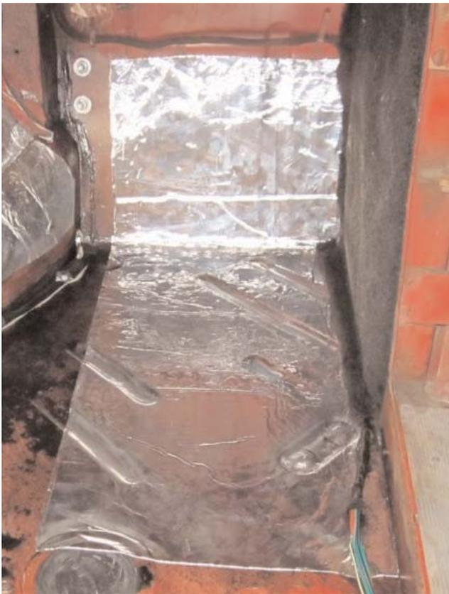
**12.** You will notice that there is a strip of floorboard between the edge of the Hushmat sheet and the transmission tunnel cover. This strip will be covered next. Gather one of the discarded pieces of wax paper backing and the black permanent marker. Lay the
