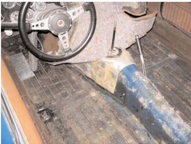
**10.** Pull up just the edge of the carpet that touches the floor on both the left and right side square frame rail at the far left and right sides of the passenger compartment. The sound deadening mat will go **UNDER** the carpet here when installed.
