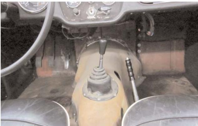
6. On our car, we removed the transmission cover from the vehicle and applied Hushmat to it. However, removing the transmission cover is unnecessary and the Hushmat can be applied with the cover still installed in the vehicle. This is the preferred method because the transmission cover is sealed to the floor which makes it difficult to remove.
