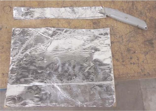
**11.** Double check the fitment of the sheet into the vehicle. Remark and recut the sheet if necessary. Then remove the wax paper backing and apply the sheet to the vehicle.
