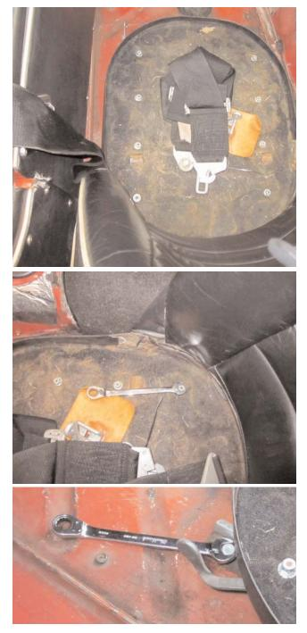
**5.** Remove the footwell rubber floor mats and footwell carpet. The carpet at the far right and left sides of the footwell will not be removed. Also remove the carpet covering the transmission cover. Note that there may be retaining snaps securing the footwell carpets. These will have to be carefully unsnapped so as not to tear the snaps out of the carpet.
