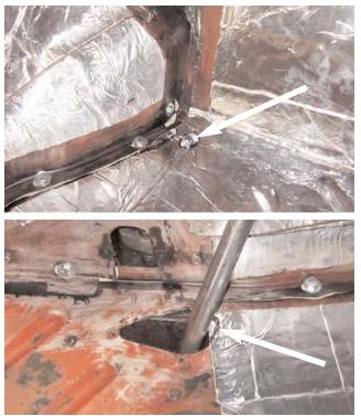
**13.** Now cover the area between the front of the seats and the sheets of Hushmat already applied to the floorboard area. Use the wax paper and the black permanent marker to draw an outline of the area onto the wax paper, cut it out, check the fitment, recut if necessary and install the sheet without the backing. Then use the black permanent marker to mark out the edge of the emergency brake handle hole, the two carpet snaps and the body drain plug hole.
