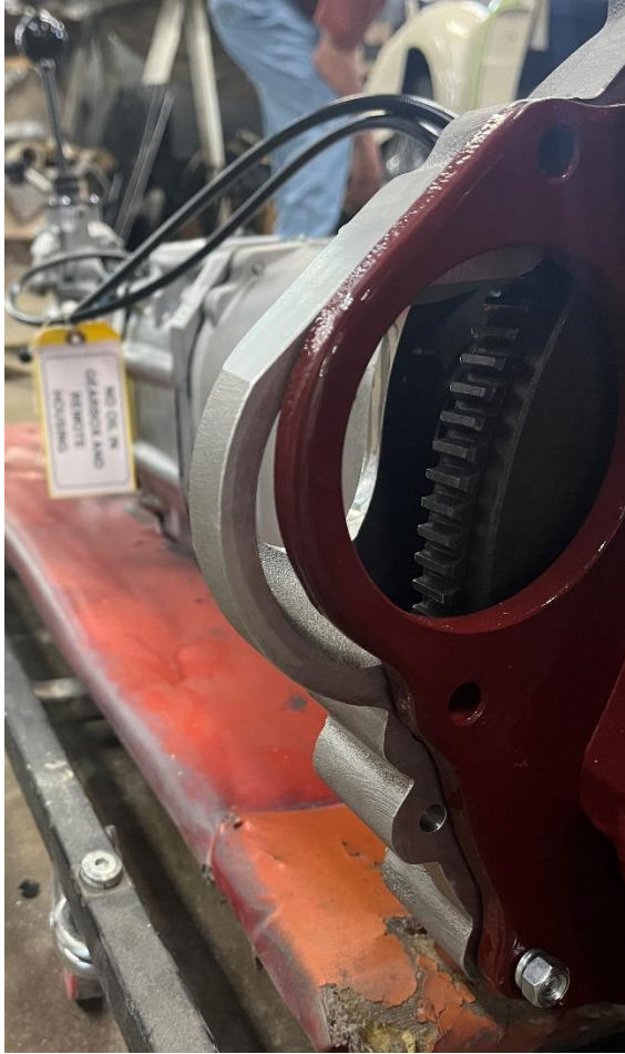
Vitesse bell housing fitted to early MGB back plate
