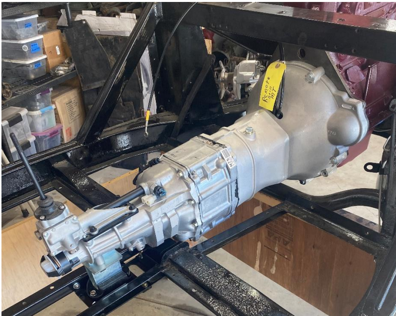
440-515 kit fitted to late MGB engine.
