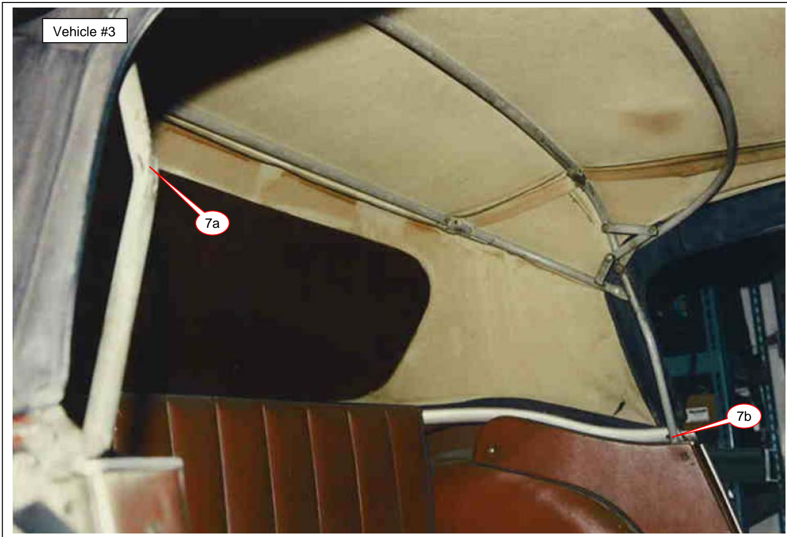
Vehicle #3: 453-675 Sliding & Folding Top Frame, as fitted to 100-6 BN4 to (CE) 68959. Note the sharp bend (7a) which is a key feature of the frame. When pulled up and locked in place, frame is right behind the B pillar (7b).
