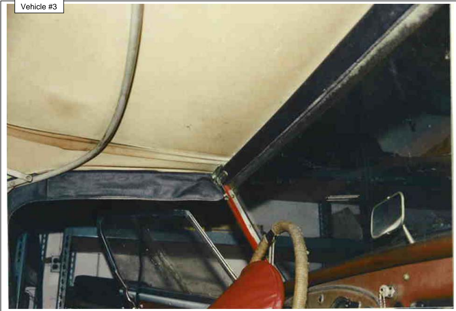
Vehicle #3: 453-675 Sliding & Folding Top Frame, as fitted to 100-6 BN4 to (CE) 68959.
