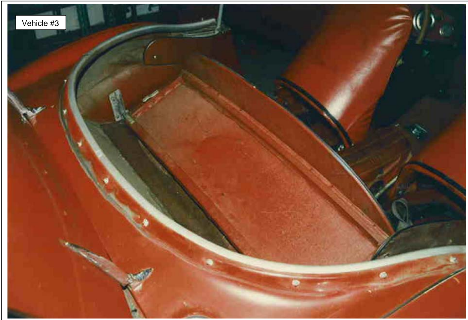
Vehicle #3: 453-675 Sliding & Folding Top Frame. Note the number and spacing of the studs for the top.
