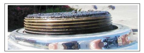
With the 280-020 O-ring fitted, install the radiator cap. Note that the o-ring in the picture above has been given a light coating of grease.
