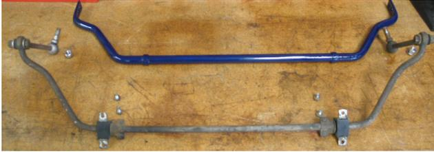
4. Gather the mounting hardware and the two anti-sway bar links provided with the new anti-sway bar. Line the items up on a work table. There should be two loosely assembled anti-sway bar links, two brackets, two polyurethane bushings, a tube of polyurethane bushing lube, four bolts, four lockwashers and four washers.
