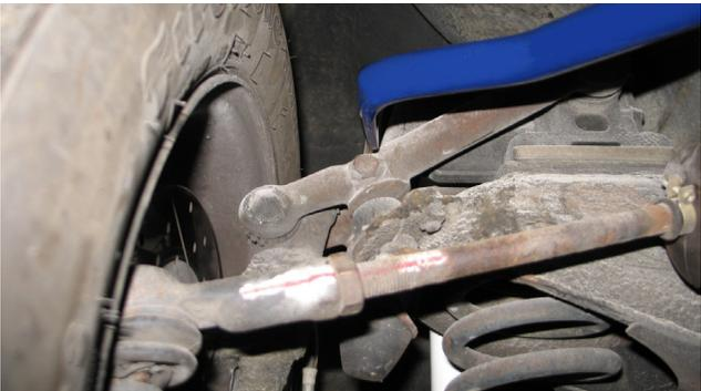
9. Remove the nut, lockwasher, washer and a-arm insert from the allen-socket headed bolt of one of the new sway bar links. Then remove the nut, two washers and lockwasher from the stud end of that new sway bar link.
