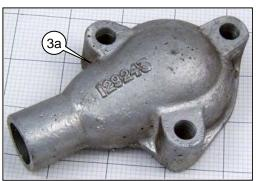
The original 12G243 thermostat housing (1a) had a distinctive "domed" top that is totally different that the "flattop" housing fitted to the 948. The original thermostat housings were not all that pretty to look at (2a) and most have suffered over the years. Dinged and/or corroded, many needed to be replaced. For the last several years, the replacement thermostat housings (3a) were not very pretty either and in addition to not fitting very well,
