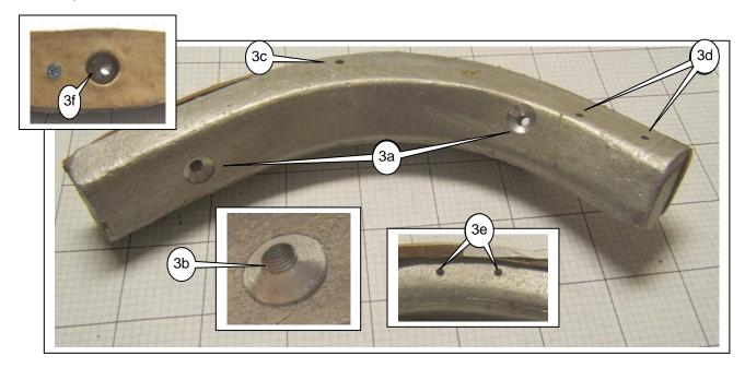
Our reproduction of the corner rails are cast aluminum, with a wooden backing strip. The holes for the two mounting screws (3a) are drilled, tapped 10-32, and counter bored for the countersunk screw heads. At the time this was being prepared, Moss did not stock a screw with those specifications.
