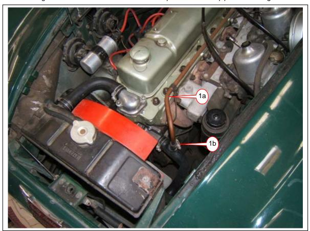
Based on the detailed study of original hoses and with the assistance of Eric Grunden (Absolutely British, Santa Maria, CA) we came up with a design that would accommodate all three applications, with some hose trimming and tweaking of the heater pipe required in some instances to achieve a proper fit. It would be nice if we could offer the three different hoses, but the demand just is not sufficient to support three different numbers.
