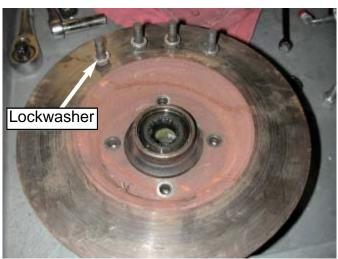
**10.** Spray brake cleaner on the rotor to clean them and to remove any rust inhibitor residue. Then place the new rotor onto the hub assembly. Thread in the four rotor mounting bolts from the previous step, each with their lockwasher. Replace them if necessary. Torque the bolts to 20 ft-lbs in a cross pattern. **Do not put the assembly back onto the spindle yet.**
