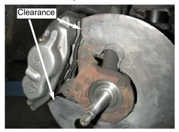
17. If the fit is satisfactory, use a 3/4 socket and ratchet to tighten the slotted nut, castle nut or locknut to 5 ft-lbs. Slacken the nut 1 flat to allow insertion of a new split pin. The required end float is 0.003 - 0.005". Fit the split pin. Half fill the hub cap with grease and fit the cap to the hub. If there is a castlenut and cotter pin instead of a locknut, install the cotter pin.
