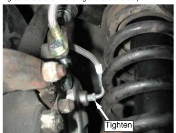
**21.** Use 1/2 and 11/16 open end wrenches to attach the far end of the brake line to the brake hard line connection at the body. Use the lockwasher from the original brake line.
