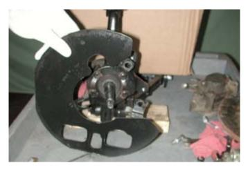
**13.** Clean/scrape the grime and grease off of the backing plate.
