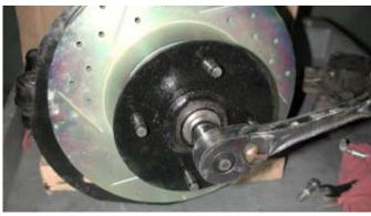
**15.** Mount the new caliper (bleeder screw goes up) onto the spindle using a provided washer on the lower bolt and the factory brake line retaining bracket on the upper bolt. The calipers are tagged left and right. Mount the brake line bracket so that it lies horizontally. Torque the mounting bolts to 60 ft-lbs with a 3/4 socket. Then tighten the brake backing plate retaining nut.
