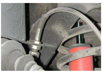
**3.** Use two 9/16 open end wrenches to loosen the fitting at the brake line retaining bracket connecting the hard brake line to the rubber brake hose.
