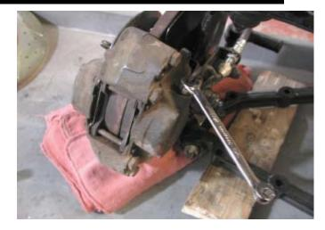
**5.** Use a 3/4 socket and a ratchet to remove the two caliper mounting bolts. Remove the bottom bolt. Then hold the caliper as you remove the upper bolt. Once the upper bolt is free of the caliper and the splash shield mount, pull the caliper from the rotor and spindle mounts. **Retrieve and keep the brake line retaining bracket and spring washers.** They will be reused.
