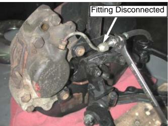
**4.** Use 9/16 and 5/8 open end wrenches to remove the soft brake line from the brake line retaining bracket. Aftermarket brake lines may require two 9/16 open end wrenches instead.
