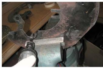
**14.** Test fit the modified backing plate and new caliper onto the spindle. Slide the backing plate onto the spindle (installation is the reverse of removal). Loosely thread on the backing plate retaining nut using a 9/16 deep socket or open end wrench. Put the rotor/hub assembly onto the spindle. Install the bearing into the hole in the hub. Slide on the bearing retaining washer and thread on the locknut (or castlenut).
