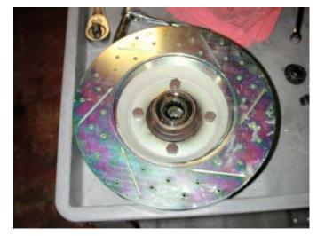
**11.** Use a 9/16 socket to remove the backing plate retaining nut and washer.
