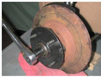
**8.** Remove the rotor/hub assembly as a unit. Remove and save the bearing and washer (they may fall out as you remove the assembly). Lay the assembly face down on the lugs. There should be a felt seal at the rear of the hub assembly (its glued on, do not remove).
