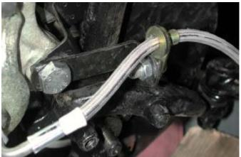
**20.** Turn the wheel all the way to the right. Position the 90 degree fitting at the caliper so that it goes between or above the coil spring. NOTE: When the suspension compresses the fitting moves outward and will remain well clear of the spring. This step makes sure it clears at full droop.
