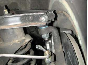
**21.** Use a 10mm combination (or a flare nut) wrench to tighten the brake line fitting at the brake caliper.
