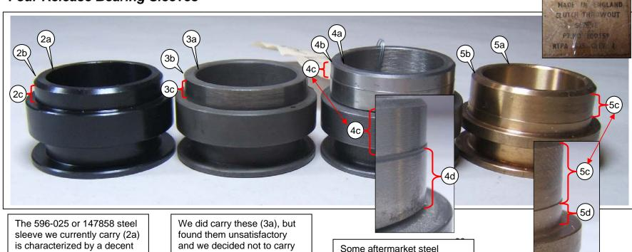
The 596-025 or 147858 steel sleeve we currently carry (2a) is characterized by a decent chamfer (2b) to facilitate pressing it into the release bearing. The area (2c) where the sleeve actually contacts the release bearing is typical at about ¼". Our sleeves follow the design of the original TR4A and TR250/6 sleeves which were identical except for the material and the hole for the pin. Our sleeves do have the hole for the anti-rotation pin used in the TR250/6.
