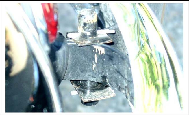
The struts were bent to bring the ends in a little, and the ends may have been trimmed to achieve the optimum fit. *If trimmed, paint the raw ends carefully with a brush to delay the formation of rust.*
