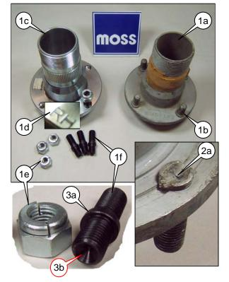
Once the peened over material is gone, the stud can be backed out fairly easily using two nuts jammed together on the front threads. In theory, there will be enough material left so you can re-use the studs. In practice, the stud is too short to double nut it and using vice-grips chews them up so badly they are pretty marginal. We strongly suggest using new studs whenever studs are removed. We also suggest using new self-locking all-metal stiff nuts (1e).
