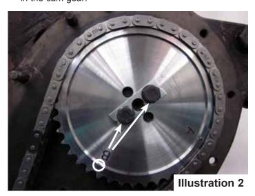
3) To check alignment of the timing gears, inspect the crank gear. Notice the tooth directly above the key on the crank is pointing straight up 12:00. Count 2 teeth clockwise on the crank gear. This is the tooth we will use to point the "B" mark at. If you were to draw an imaginary line from the center of the crankshaft to the center of the camshaft, the 2nd tooth on the crank gear and the "B" mark on the cam gear would fall on this
