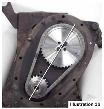
4) Once proper alignment has been achieved, follow the manual to reassemble your engine. Don't forget to properly torque the cam gear to the cam and use appropriate lock tab.
