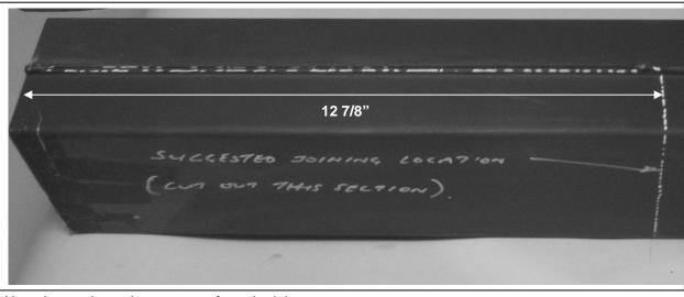
Note the section to be cut out to form the joint.
