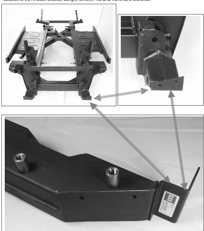
The tubes have been placed into the holes for reference only; they are sticking out too far and should not look like this when they are welded in place.
