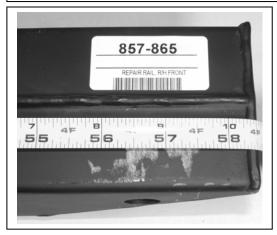
The frame rail repair section is about 58 ½" long. Included with the frame rail are the two threaded tubes that go through the rail at the front, and the AH505R bracket for attaching the shroud.
