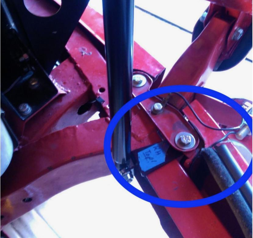
3. On the bonnet, place a Fender Washer on a Ball Stud and see if you can thread it through the existing hole from the inside of the wheel well as shown in the next photo. If you cannot, you may have to run a 5/16" drill bit through the hole to remove a sliver of paint thickness.
