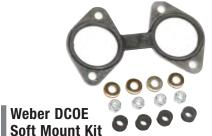
Vibration wreaks havoc with fuel flow. A Weber DCOE soft mount kit helps dampen these vibrations by isolating the carburetor from the manifold, and improves carburetor efficiency.
