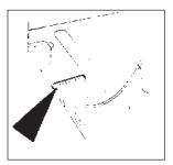
**Body Serial Number (TR4-4A)** On right firewall "shelf" by voltage regulator.
