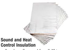
Install on doors, floors, and firewall. This insulation consists of an 80 mil thick butyl rubber-core covered with a 2.4 mil aluminum coating. It deadens body panel vibrations and reduces heat transfer. The kit contains nine 29" x 20" sheets (36 sq ft).
