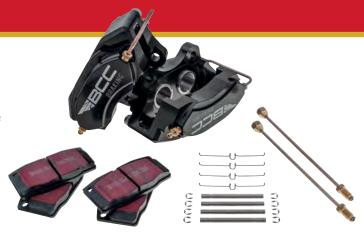
Please Note: Always use the new caliper to hose link pipes provided. These calipers are manufactured with imperial threads. When fitting to a TR6 with metric calipers please ensure that the brake hose to caliper pipe supplied is used.
