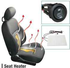
A little warmth in the right place can really make driving a much more comfortable experience. This therapeutic seat-heater has dual zones and two settings to keep your seat and lower back toasty. Designed to be installed under existing upholstery or seat covers, this kit is suitable for alternator equipped cars. Sold as a set for one seat. Negative ground cars with an alternator only.
