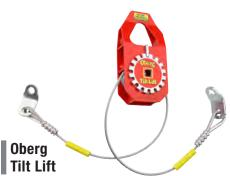
Allows easy adjustment of an engine's lift angle through a full 90° of movement. Adjust with ½" ratchet; 2,000 lb capacity with a 3:1 safety load factor. A positive lock ensures the engine stays put. All steel construction and small size.
